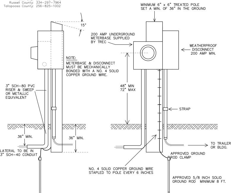
This drawing shows one of many acceptable configurations for meterbase & disconnect configuration. Other alignments include: Meterbase above disconnect (offset for service riser conduit), Meterbase with disconnect on back side of pole, etc.
