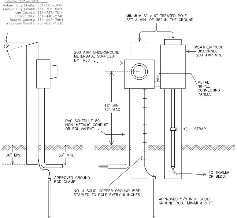
This drawing shows one of many acceptable configurations for meterbase & disconnect configuration. Other alignments include: Meterbase above disconnect (offset for service riser conduit), Meterbase with disconnect on back side of pole, etc.
